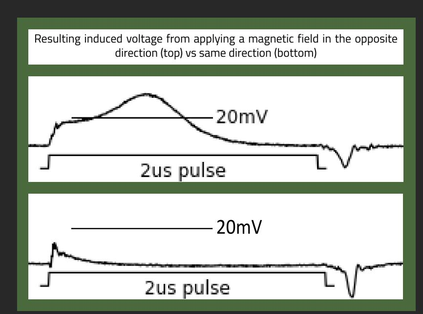
The **switching** of the core's magnetic field can induce a small number of volts into a **second** wire, called a **sense** wire. This only occurs when the core **changes** states. Using this property, we can set a core to a **known** value, normally 0, then test for a response. If we detect a **change**, we know that the core went from a non-0 state to 0, so the core **was a 1**. **One** sense wire can be used for **all** cores.
